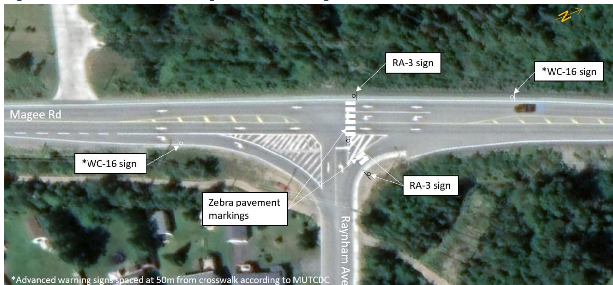
Figure 5 - Recommended Crossing Treatment on Magee Road
