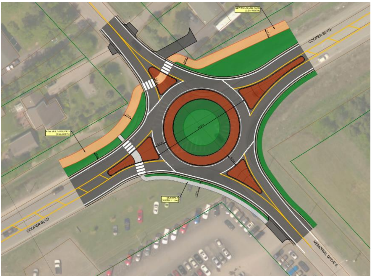
Figure 7 - Memorial Drive at Cooper Boulevard Roundabout Concept
